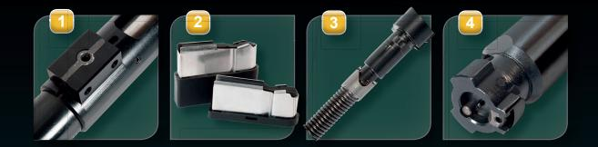
**1** The barrel is manufactured from specialist gun barrel steel and fitted in the actioncasing with a recoil bed. This technology allows for an interchangeable barrel system, which in turn allows the hunter to change caliber for different quarry species. A great plus point for the hunter, who may want to use the same weapon for both hunting from a hide and tracking.
